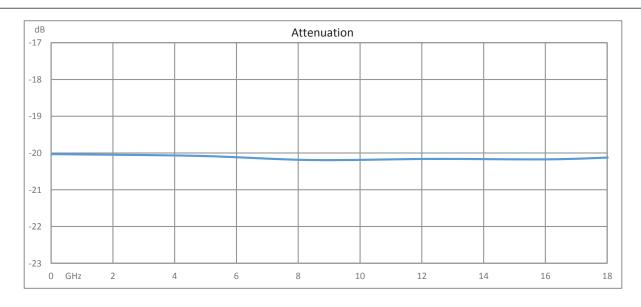
20 dB Fixed Attenuator SMA Male (Plug) to SMA Female (Jack) Up to 18 GHz Rated to 2 Watts, Passivated Stainless Steel Body, 1.35 VSWR from Fairview Microwave is in-stock and available to ship same-day. All of our RF/microwave products are available off-the-shelf from our ISO 9001:2008 certified facilities in Lewisville, Texas. Fairview Microwave is RF on-demand.
