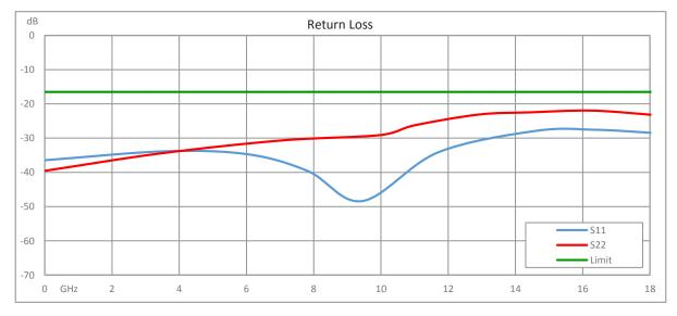
30 dB Fixed Attenuator SMA Male (Plug) to SMA Female (Jack) Up to 18 GHz Rated to 2 Watts, Passivated Stainless Steel Body, 1.35 VSWR
