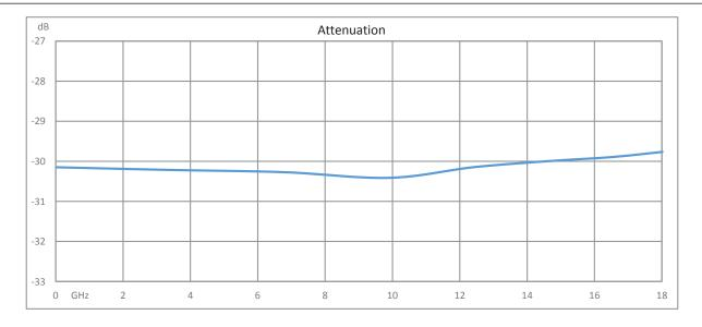
30 dB Fixed Attenuator SMA Male (Plug) to SMA Female (Jack) Up to 18 GHz Rated to 2 Watts, Passivated Stainless Steel Body, 1.35 VSWR from Fairview Microwave is in-stock and available to ship same-day. All of our RF/microwave products are available off-the-shelf from our ISO 9001:2008 certified facilities in Lewisville, Texas. Fairview Microwave is RF on-demand.
