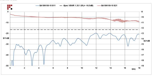
10 dB Fixed Attenuator N Male (Plug) to N Female (Jack) Directional Up to 18 GHz Rated to 100 Watts, Heatsink Body, 1.35 VSWR from Fairview Microwave is in-stock and available to ship same-day. All of our RF/microwave products are available off-the-shelf from our ISO 9001:2008 certified facilities in Lewisville, Texas. Fairview Microwave is RF on-demand.
