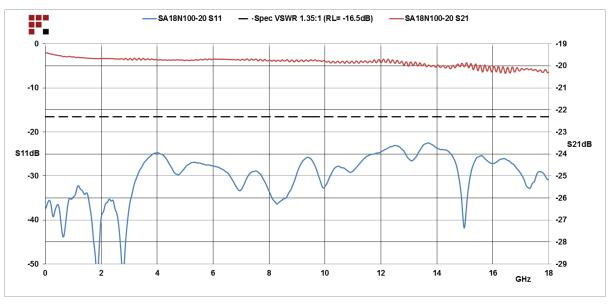
20 dB Fixed Attenuator N Male (Plug) to N Female (Jack) Directional Up to 18 GHz Rated to 100 Watts, Heatsink Body, 1.35 VSWR from Fairview Microwave is in-stock and available to ship same-day. All of our RF/microwave products are available off-the-shelf from our ISO 9001:2008 certified facilities in Lewisville, Texas. Fairview Microwave is RF on-demand.
