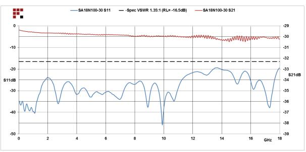
30 dB Fixed Attenuator N Male (Plug) to N Female (Jack) Directional Up to 18 GHz Rated to 100 Watts, Heatsink Body, 1.35 VSWR from Fairview Microwave is in-stock and available to ship same-day. All of our RF/microwave products are available off-the-shelf from our ISO 9001:2008 certified facilities in Lewisville, Texas. Fairview Microwave is RF on-demand.
