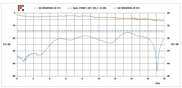
30 dB Fixed Attenuator N Male (Plug) to N Female (Jack) Directional Up to 18 GHz Rated to 200 Watts, Heatsink Body, 1.5 VSWR from Fairview Microwave is in-stock and available to ship same-day. All of our RF/microwave products are available off-the-shelf from our ISO 9001:2008 certified facilities in Lewisville, Texas. Fairview Microwave is RF on-demand.
