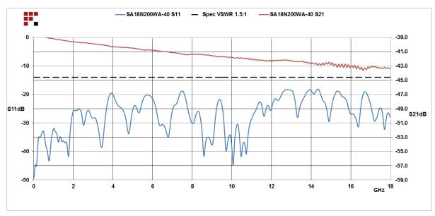
40 dB Fixed Attenuator N Male (Plug) to N Female (Jack) Directional Up to 18 GHz Rated to 200 Watts, Heatsink Body, 1.5 VSWR from Fairview Microwave is in-stock and available to ship same-day. All of our RF/microwave products are available off-the-shelf from our ISO 9001:2008 certified facilities in Lewisville, Texas. Fairview Microwave is RF on-demand.
