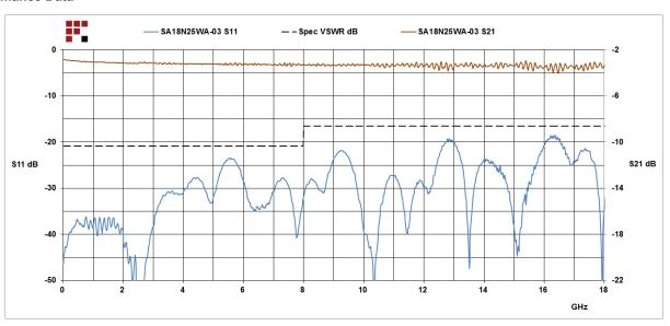
3 dB Fixed Attenuator N Male (Plug) to N Female (Jack) Up to 18 GHz Rated to 25 Watts, Heatsink Body, 1.35 VSWR from Fairview Microwave is in-stock and available to ship same-day. All of our RF/microwave products are available off-the-shelf from our ISO 9001:2008 certified facilities in Lewisville, Texas. Fairview Microwave is RF on-demand.
