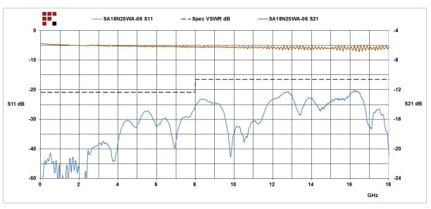
6 dB Fixed Attenuator N Male (Plug) to N Female (Jack) Up to 18 GHz Rated to 25 Watts, Heatsink Body, 1.35 VSWR from Fairview Microwave is in-stock and available to ship same-day. All of our RF/microwave products are available off-the-shelf from our ISO 9001:2008 certified facilities in Lewisville, Texas. Fairview Microwave is RF on-demand.
