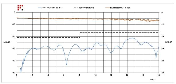
10 dB Fixed Attenuator N Male (Plug) to N Female (Jack) Up to 18 GHz Rated to 25 Watts, Heatsink Body, 1.35 VSWR from Fairview Microwave is in-stock and available to ship same-day. All of our RF/microwave products are available off-the-shelf from our ISO 9001:2008 certified facilities in Lewisville, Texas. Fairview Microwave is RF on-demand.
