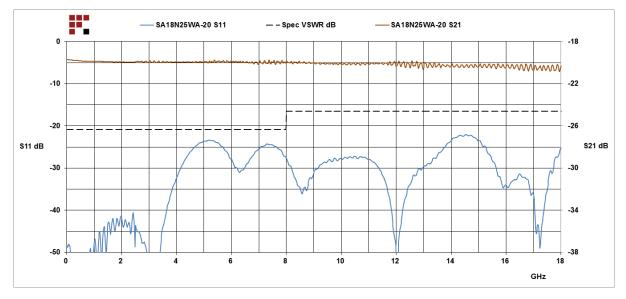
20 dB Fixed Attenuator N Male (Plug) to N Female (Jack) Up to 18 GHz Rated to 25 Watts, Heatsink Body, 1.35 VSWR from Fairview Microwave is in-stock and available to ship same-day. All of our RF/microwave products are available off-the-shelf from our ISO 9001:2008 certified facilities in Lewisville, Texas. Fairview Microwave is RF on-demand.
