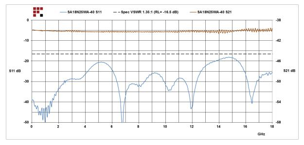
40 dB Fixed Attenuator N Male (Plug) to N Female (Jack) Up to 18 GHz Rated to 25 Watts, Heatsink Body, 1.35 VSWR from Fairview Microwave is in-stock and available to ship same-day. All of our RF/microwave products are available off-the-shelf from our ISO 9001:2008 certified facilities in Lewisville, Texas. Fairview Microwave is RF on-demand.
