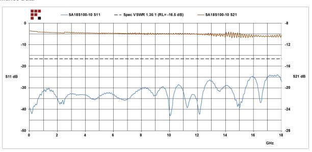
10 dB Fixed Attenuator SMA Male (Plug) to SMA Female (Jack) Directional Up to 18 GHz Rated to 100 Watts, Heatsink Body, 1.35 VSWR from Fairview Microwave is in-stock and available to ship same-day. All of our RF/microwave products are available off-the-shelf from our ISO 9001:2008 certified facilities in Lewisville, Texas. Fairview Microwave is RF on-demand.
