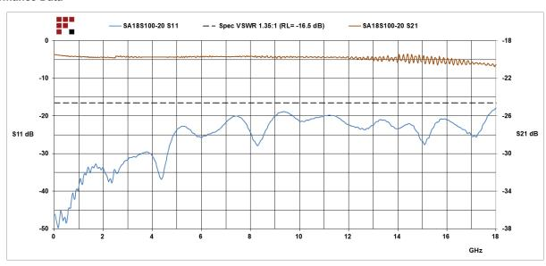
20 dB Fixed Attenuator SMA Male (Plug) to SMA Female (Jack) Directional Up to 18 GHz Rated to 100 Watts, Heatsink Body, 1.35 VSWR from Fairview Microwave is in-stock and available to ship same-day. All of our RF/microwave products are available off-the-shelf from our ISO 9001:2008 certified facilities in Lewisville, Texas. Fairview Microwave is RF on-demand.
