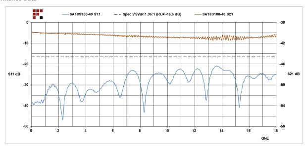
40 dB Fixed Attenuator SMA Male (Plug) to SMA Female (Jack) Directional Up to 18 GHz Rated to 100 Watts, Heatsink Body, 1.35 VSWR from Fairview Microwave is in-stock and available to ship same-day. All of our RF/microwave products are available off-the-shelf from our ISO 9001:2008 certified facilities in Lewisville, Texas. Fairview Microwave is RF on-demand.
