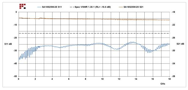
20 dB Fixed Attenuator SMA Male (Plug) to SMA Female (Jack) Up to 18 GHz Rated to 25 Watts, Heatsink Body, 1.35 VSWR
