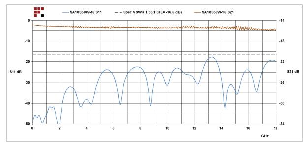
15 dB Fixed Attenuator SMA Male (Plug) to SMA Female (Jack) Up to 18 GHz Rated to 50 Watts, Heatsink Body, 1.35 VSWR
