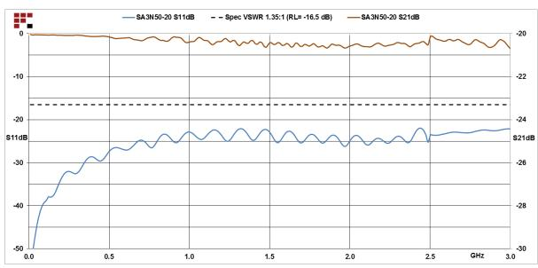
20 dB Fixed Attenuator N Male (Plug) to N Female (Jack) Up to 3 GHz Rated to 50 Watts, Heatsink Body, 1.35 VSWR from Fairview Microwave is in-stock and available to ship same-day. All of our RF/microwave products are available off-the-shelf from our ISO 9001:2008 certified facilities in Lewisville, Texas. Fairview Microwave is RF on-demand.
