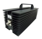
3 dB Fixed Attenuator N Male (Plug) to N Female (Jack) Directional Up to 3 GHz Rated to 500 Watts, Heatsink Body, 1.4 VSWR from Fairview Microwave is in-stock and available to ship same-day. All of our RF/microwave products are available off-the-shelf from our ISO 9001:2008 certified facilities in Lewisville, Texas. Fairview Microwave is RF on-demand.
