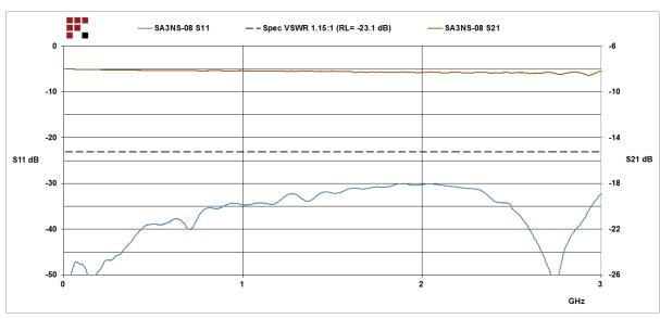
8 dB Fixed Attenuator N Male (Plug) To N Female (Jack) Up To 3 GHz Rated To 2 Watts, Brass Tri-Metal Body, 1.15 VSWR from Fairview Microwave is in-stock and available to ship same-day. All of our RF/microwave products are available off-the-shelf from our ISO 9001:2008 certified facilities in Lewisville, Texas. Fairview Microwave is RF on-demand.
