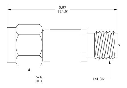
REVERSE POLARITY SMA MALE REVERSE POLARITY SMA FEMALE
