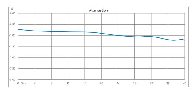
1 dB Fixed Attenuator 2.92mm Male (Plug) to 2.92mm Female (Jack) Up to 40 GHz Rated to 0.5 Watts, Passivated Stainless Steel Body, 1.5 VSWR from Fairview Microwave is in-stock and available to ship same-day. All of our RF/microwave products are available off-the-shelf from our ISO 9001:2008 certified facilities in Lewisville, Texas. Fairview Microwave is RF on-demand.
