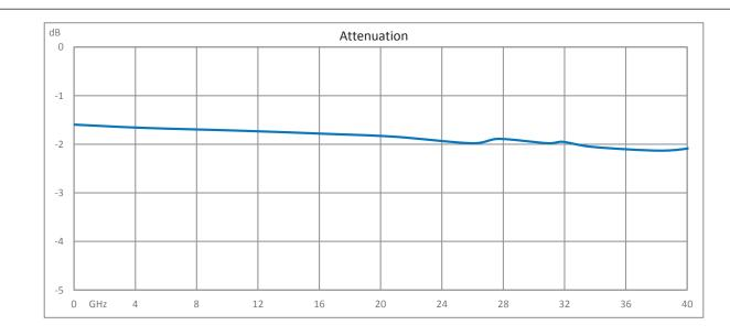
2 dB Fixed Attenuator 2.92mm Male (Plug) to 2.92mm Female (Jack) Up to 40 GHz Rated to 0.5 Watts, Passivated Stainless Steel Body, 1.5 VSWR from Fairview Microwave is in-stock and available to ship same-day. All of our RF/microwave products are available off-the-shelf from our ISO 9001:2008 certified facilities in Lewisville, Texas. Fairview Microwave is RF on-demand.
