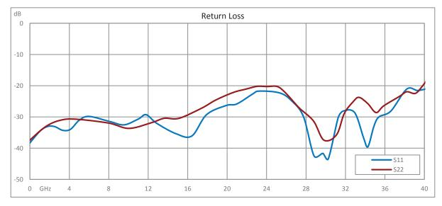
2 dB Fixed Attenuator 2.92mm Male (Plug) to 2.92mm Female (Jack) Up to 40 GHz Rated to 0.5 Watts, Passivated Stainless Steel Body, 1.5 VSWR
