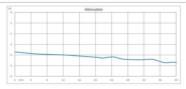
4 dB Fixed Attenuator 2.92mm Male (Plug) to 2.92mm Female (Jack) Up to 40 GHz Rated to 0.5 Watts, Passivated Stainless Steel Body, 1.5 VSWR from Fairview Microwave is in-stock and available to ship same-day. All of our RF/microwave products are available off-the-shelf from our ISO 9001:2008 certified facilities in Lewisville, Texas. Fairview Microwave is RF on-demand.
