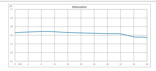
20 dB Fixed Attenuator 2.92mm Male (Plug) to 2.92mm Female (Jack) Up to 40 GHz Rated to 0.5 Watts, Passivated Stainless Steel Body, 1.5 VSWR from Fairview Microwave is in-stock and available to ship same-day. All of our RF/microwave products are available off-the-shelf from our ISO 9001:2008 certified facilities in Lewisville, Texas. Fairview Microwave is RF on-demand.
