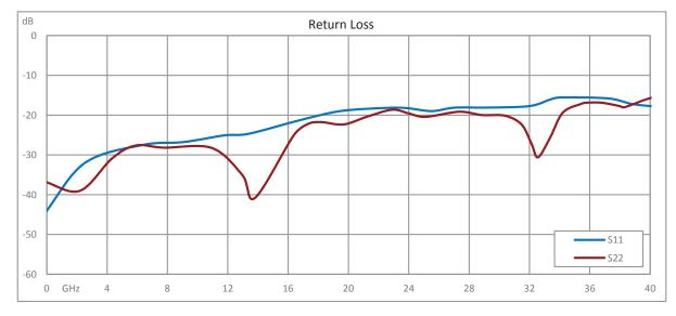
20 dB Fixed Attenuator 2.92mm Male (Plug) to 2.92mm Female (Jack) Up to 40 GHz Rated to 0.5 Watts, Passivated Stainless Steel Body, 1.5 VSWR
