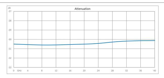
30 dB Fixed Attenuator 2.92mm Male (Plug) to 2.92mm Female (Jack) Up to 40 GHz Rated to 0.5 Watts, Passivated Stainless Steel Body, 1.5 VSWR from Fairview Microwave is in-stock and available to ship same-day. All of our RF/microwave products are available off-the-shelf from our ISO 9001:2008 certified facilities in Lewisville, Texas. Fairview Microwave is RF on-demand.
