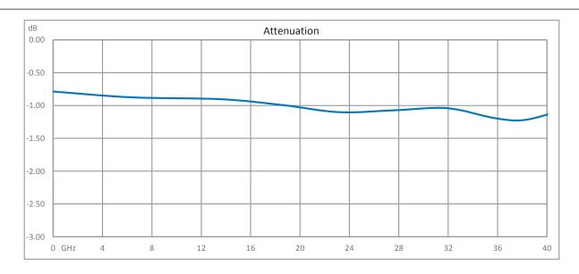
1 dB Fixed Attenuator 2.92mm Male (Plug) to 2.92mm Female (Jack) Up to 40 GHz Rated to 1 Watt, Passivated Stainless Steel Body, 1.4 VSWR from Fairview Microwave is in-stock and available to ship same-day. All of our RF/microwave products are available off-the-shelf from our ISO 9001:2008 certified facilities in Lewisville, Texas. Fairview Microwave is RF on-demand.
