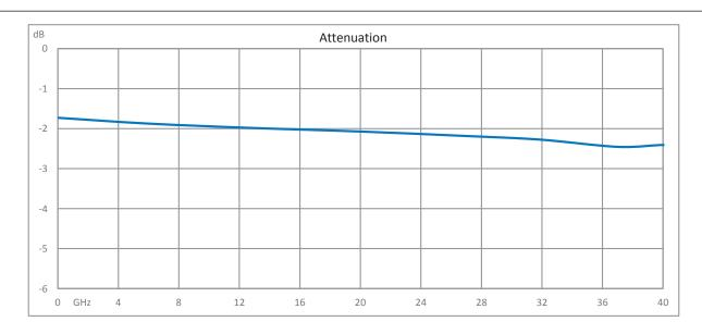
2 dB Fixed Attenuator 2.92mm Male (Plug) to 2.92mm Female (Jack) Up to 40 GHz Rated to 1 Watt, Passivated Stainless Steel Body, 1.4 VSWR from Fairview Microwave is in-stock and available to ship same-day. All of our RF/microwave products are available off-the-shelf from our ISO 9001:2008 certified facilities in Lewisville, Texas. Fairview Microwave is RF on-demand.
