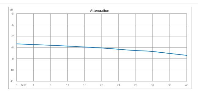
8 dB Fixed Attenuator 2.92mm Male (Plug) to 2.92mm Female (Jack) Up to 40 GHz Rated to 1 Watt, Passivated Stainless Steel Body, 1.4 VSWR from Fairview Microwave is in-stock and available to ship same-day. All of our RF/microwave products are available off-the-shelf from our ISO 9001:2008 certified facilities in Lewisville, Texas. Fairview Microwave is RF on-demand.
