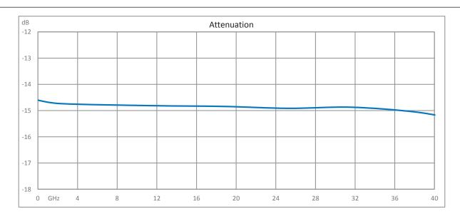
15 dB Fixed Attenuator 2.92mm Male (Plug) to 2.92mm Female (Jack) Up to 40 GHz Rated to 1 Watt, Passivated Stainless Steel Body, 1.4 VSWR from Fairview Microwave is in-stock and available to ship same-day. All of our RF/microwave products are available off-the-shelf from our ISO 9001:2008 certified facilities in Lewisville, Texas. Fairview Microwave is RF on-demand.
