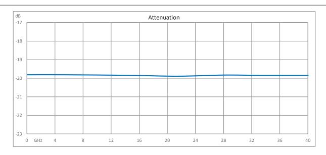
20 dB Fixed Attenuator 2.92mm Male (Plug) to 2.92mm Female (Jack) Up to 40 GHz Rated to 1 Watt, Passivated Stainless Steel Body, 1.4 VSWR from Fairview Microwave is in-stock and available to ship same-day. All of our RF/microwave products are available off-the-shelf from our ISO 9001:2008 certified facilities in Lewisville, Texas. Fairview Microwave is RF on-demand.
