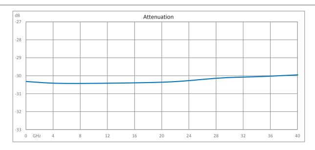
30 dB Fixed Attenuator 2.92mm Male (Plug) to 2.92mm Female (Jack) Up to 40 GHz Rated to 1 Watt, Passivated Stainless Steel Body, 1.4 VSWR from Fairview Microwave is in-stock and available to ship same-day. All of our RF/microwave products are available off-the-shelf from our ISO 9001:2008 certified facilities in Lewisville, Texas. Fairview Microwave is RF on-demand.
