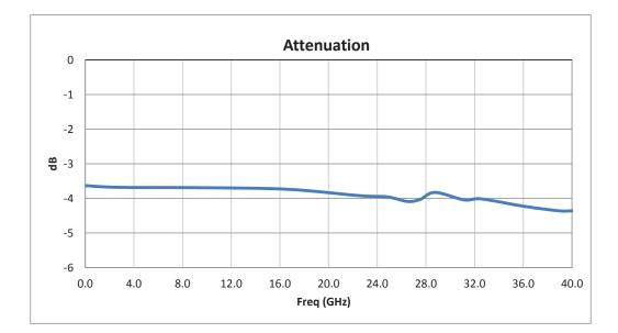
4 dB Fixed Attenuator 2.92mm Male (Plug) to 2.92mm Female (Jack) Up to 40 GHz Rated to 2 Watts, Passivated Stainless Steel Body, 1.4 VSWR
