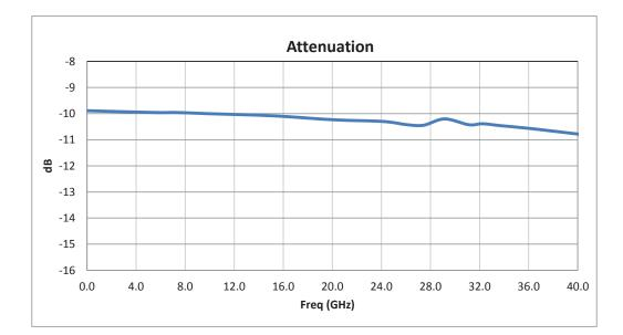
10 dB Fixed Attenuator 2.92mm Male (Plug) to 2.92mm Female (Jack) Up to 40 GHz Rated to 2 Watts, Passivated Stainless Steel Body, 1.4 VSWR
