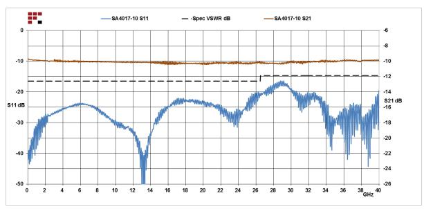
10 dB Fixed Attenuator 2.92mm Male (Plug) to 2.92mm Female (Jack) Up to 40 GHz Rated to 5 Watts, Heatsink Body, 1.45 VSWR from Fairview Microwave is in-stock and available to ship same-day. All of our RF/microwave products are available off-the-shelf from our ISO 9001:2008 certified facilities in Lewisville, Texas. Fairview Microwave is RF on-demand.
