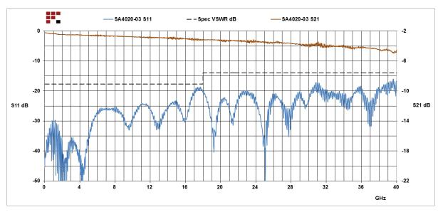
3 dB Fixed Attenuator 2.92mm Male (Plug) to 2.92mm Female (Jack) Up to 40 GHz Rated to 10 Watts, Heatsink Body, 1.4 VSWR from Fairview Microwave is in-stock and available to ship same-day. All of our RF/microwave products are available off-the-shelf from our ISO 9001:2008 certified facilities in Lewisville, Texas. Fairview Microwave is RF on-demand.
