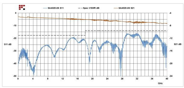
6 dB Fixed Attenuator 2.92mm Male (Plug) to 2.92mm Female (Jack) Up to 40 GHz Rated to 10 Watts, Heatsink Body, 1.4 VSWR from Fairview Microwave is in-stock and available to ship same-day. All of our RF/microwave products are available off-the-shelf from our ISO 9001:2008 certified facilities in Lewisville, Texas. Fairview Microwave is RF on-demand.
