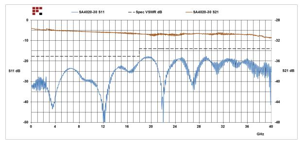
30 dB Fixed Attenuator 2.92mm Male (Plug) to 2.92mm Female (Jack) Directional Up to 40 GHz Rated to 10 Watts, Heatsink Body, 1.4 VSWR from Fairview Microwave is in-stock and available to ship same-day. All of our RF/microwave products are available off-the-shelf from our ISO 9001:2008 certified facilities in Lewisville, Texas. Fairview Microwave is RF on-demand.
