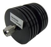
30 dB Fixed Attenuator 2.92mm Male (Plug) to 2.92mm Female (Jack) Directional Up to 40 GHz Rated to 10 Watts, Heatsink Body, 1.4 VSWR
