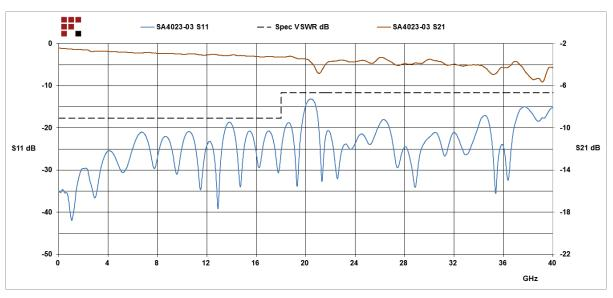
3 dB Fixed Attenuator 2.92mm Male (Plug) to 2.92mm Female (Jack) Directional Up to 40 GHz Rated to 20 Watts, Heatsink Body, 1.5 VSWR from Fairview Microwave is in-stock and available to ship same-day. All of our RF/microwave products are available off-the-shelf from our ISO 9001:2008 certified facilities in Lewisville, Texas. Fairview Microwave is RF on-demand.
