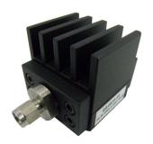
10 dB Fixed Attenuator SMA Male (Plug) to SMA Female (Jack) Up to 4 GHz Rated to 25 Watts, Heatsink Body, 1.2 VSWR from Fairview Microwave is in-stock and available to ship same-day. All of our RF/microwave products are available off-the-shelf from our ISO 9001:2008 certified facilities in Lewisville, Texas. Fairview Microwave is RF on-demand.
