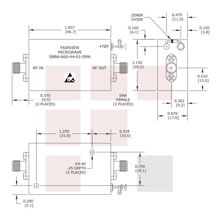
NOTE: HEAT SINK REQUIRED FOR PROPER OPERATION, UNIT IS COOLED BY CONDUCTING TO HEAT SINK.
