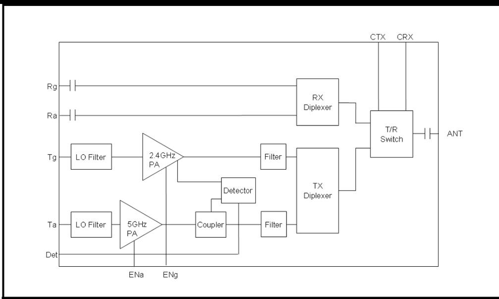
**Figure 1: SE2548A Functional Block Diagram**
