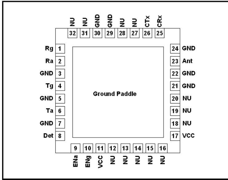
Figure 2: SE2548A Pin Out (Top View Through Package)
