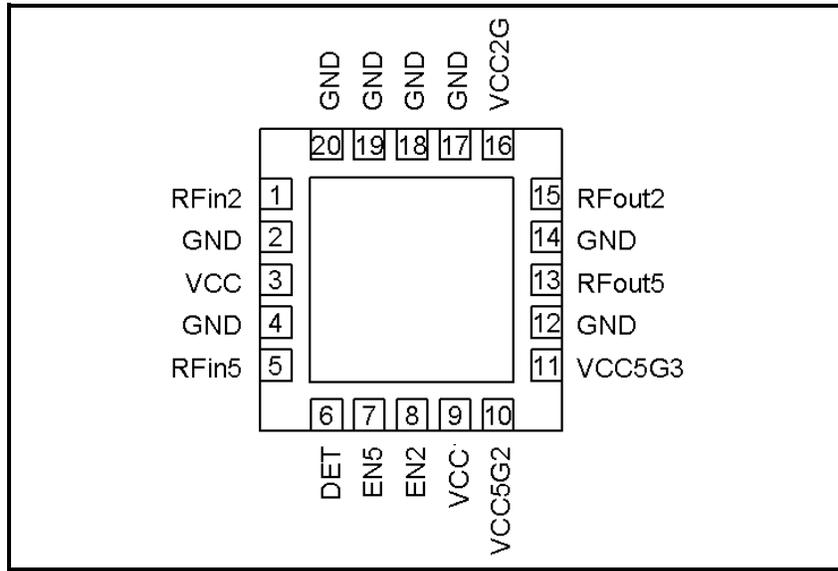
**Figure 2: SE2580L Pin Out (Top View Through Package)**
