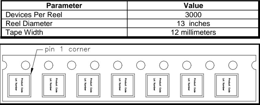
**Figure 9: Detailed Tape and Reel Information (All dimensions in Millimeters)**
