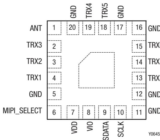
Figure 2. SKY13561-670LF Pinout – 20-Pin QFN (Top View)
