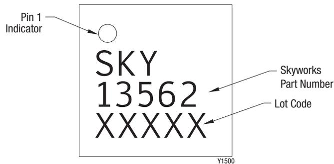
**Figure 10. Typical Part Markings (Top View)**
