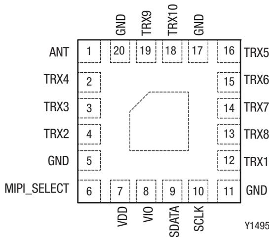
**Figure 2. SKY13562-670LF Pinout – 20-Pin QFN (Top View)**
