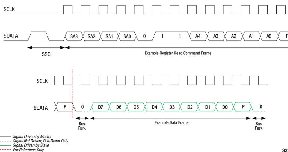
**Figure 5. Register Read Command Timing Diagram**
