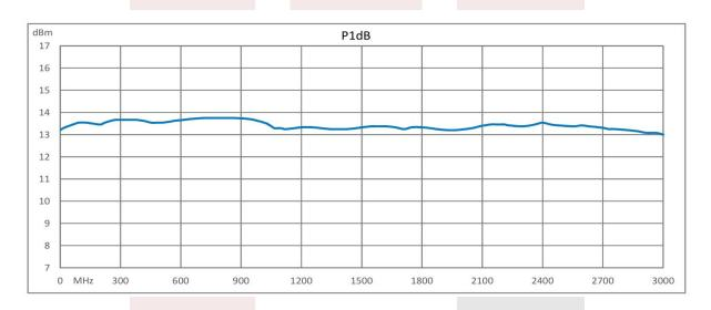
1.6 dB NF Low Noise Amplifier, Operating From 20 MHz to 3 GHz with 25 dB Gain, 13.5 dBm P1dB and SMA from Fairview Microwave is in-stock and available to ship same-day. All of our RF/microwave products are available off-the-shelf from our ISO 9001:2008 certified facilities in Lewisville, Texas. Fairview Microwave is RF on-demand.
