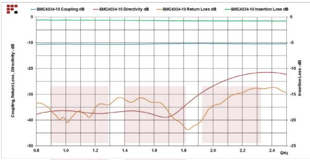
N Directional Coupler 10 dB Coupled Port From 800 MHz to 2.5 GHz Rated To 60 Watts from Fairview Microwave is in-stock and available to ship same-day. All of our RF/microwave products are available off-the-shelf from our ISO 9001:2008 certified facilities in Allen, Texas. Fairview Microwave is RF on-demand.
