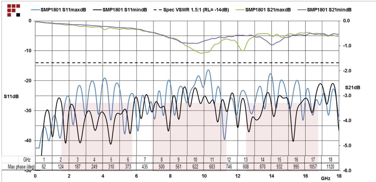
SMA Variable Phase Shifter With an Adjustable Phase of 60 Deg. Per GHz and From DC to 18 GHz from Fairview Microwave is in-stock and available to ship same-day. All of our RF/microwave products are available off-the-shelf from our ISO 9001:2008 certified facilities in Lewisville, Texas. Fairview Microwave is RF on-demand.
