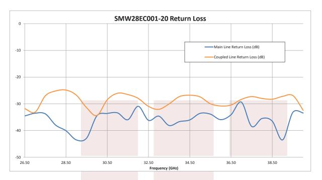
WR-28 Directional Waveguide Coupler 20 dB With UG-599/U Flange and E-Plane Coupled Port From 26.5 GHz to 40 GHz Ka Band from Fairview Microwave is in-stock and available to ship same-day. All of our RF/microwave products are available off-the-shelf from our ISO 9001:2008 certified facilities in Allen, Texas. Fairview Microwave is RF on-demand.
