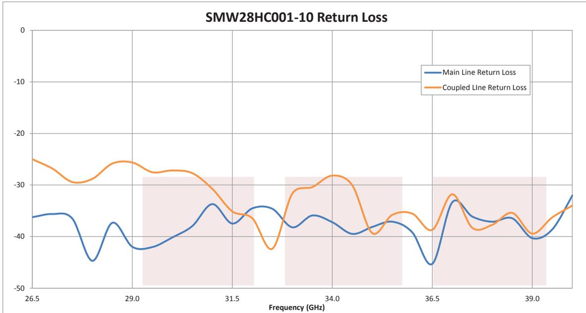
10 dB WR-28 Waveguide Broadwall Coupler with UG-599/U Square Cover Flange and H-Plane Coupled Port from 26.5 GHz to 40 GHz in Brass Copper from Fairview Microwave is in-stock and available to ship same-day. All of our RF/microwave products are available off-the-shelf from our ISO 9001:2008 certified facilities in Lewisville, Texas. Fairview Microwave is RF on-demand.
